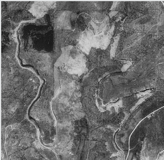
Pre-SMCRA abandoned site with highwalls, pits, and unreclaimed spoil.
