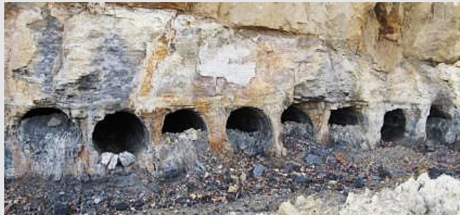
Bank of legacy auger holes in Gallia County, Ohio.
