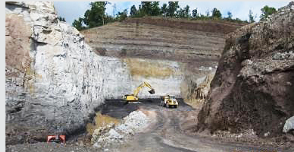
B&N Coal Company daylighting of legacy auger mines at its remining operation in Noble County, Ohio.
